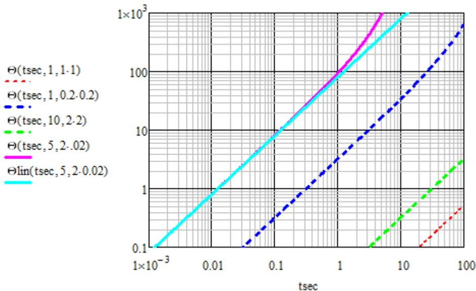
**Figure 1:** “Onderdonk solutions” of an insulated wire: temperature rise (K) vs. time (s). The pink line represents any ( $A=0.04$  mm<sup>2</sup>) wire with 5 Amps.
