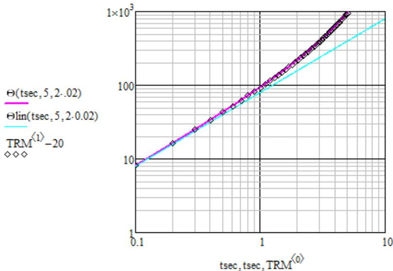
**Figure 2:** Numerical simulation of a heated and insulated wire with TRM (symbols) vs. analytic solution (pink line= Eq.(7)) for 5 Amps and cross-section 0.04 mm<sup>2</sup>.
