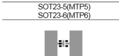
Figure 14: „Cu-foil“ applied by NJR in a test board
